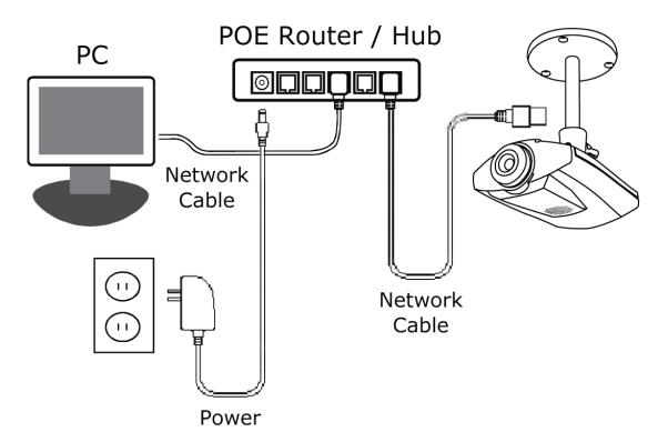
When your router / hub doesn't support POE connection (An optional POE connected required)
